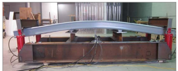
8" thick specimen at full cylinder travel
