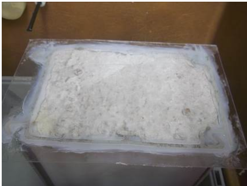
Photo No. 2 Sheathed Specimen in Salt Fog Exposure Chamber
