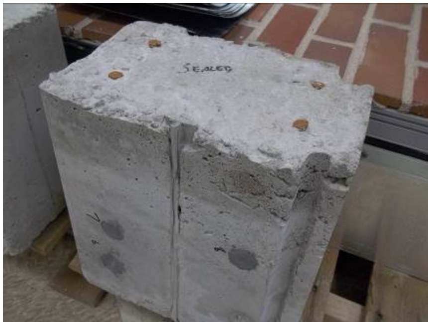
Photo No. 8 Truline System Sheathed Specimen (Sealed Joint) - Post Test Condition
