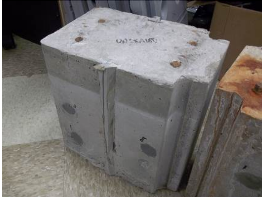
Photo No. 7 Truline System Sheathed Specimen (Unsealed Joint) - Post Test Condition
