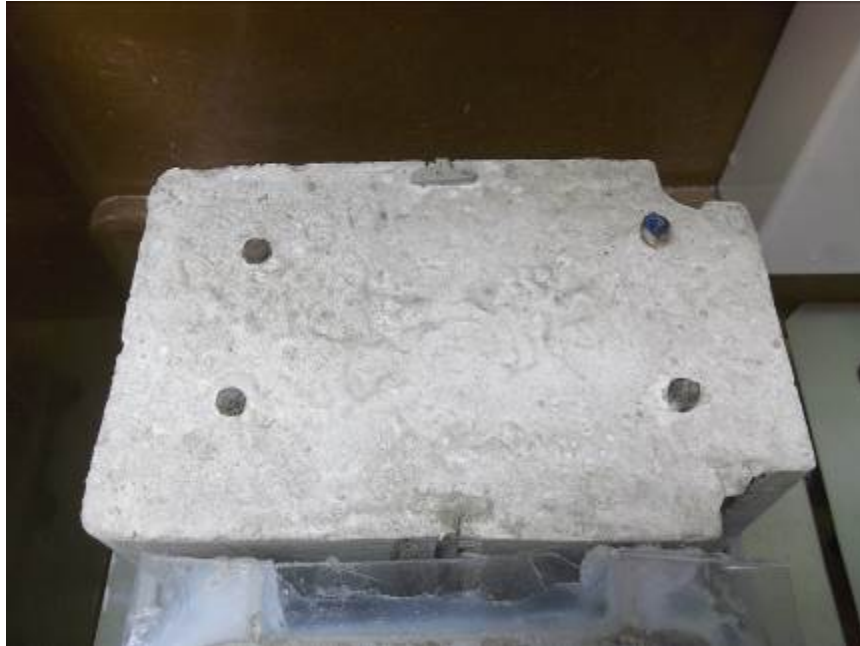
Photo No. 1 Full-Exposure Specimen in Salt Fog Exposure Chamber
