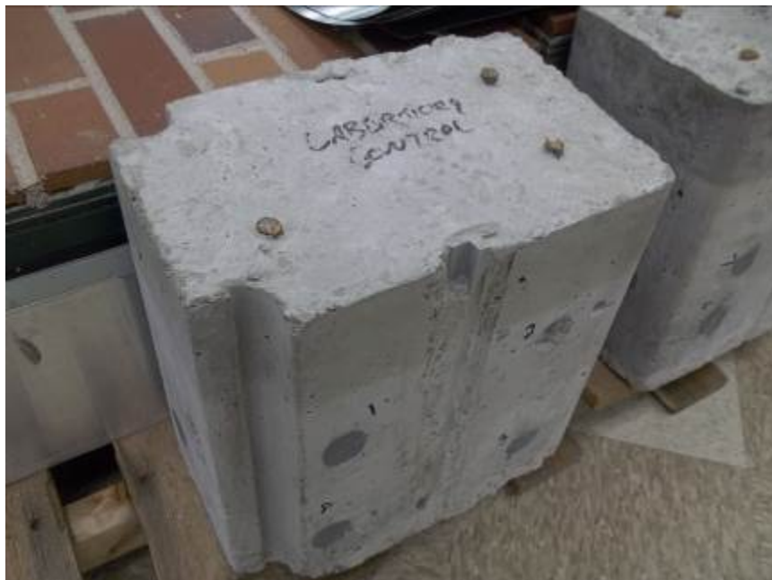
Photo No. 6 Laboratory Conditioned (Unexposed) Control Specimen
