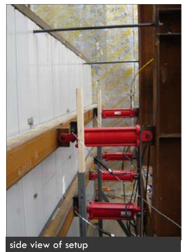
hydraulic cylinders and transducers
