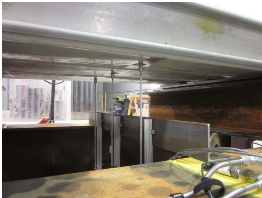
Photo No. 2 Bottom Center of Test Specimen showing LVDT locations
