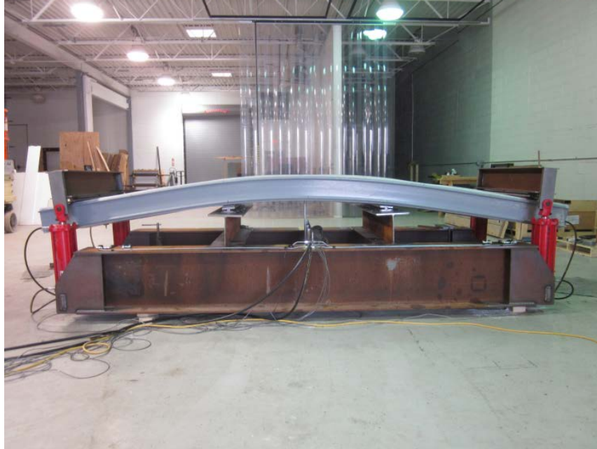
Photo No. 3 Typical 8" Thick Specimen at Full Cylinder Travel
