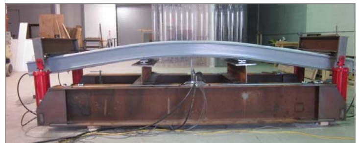
8" thick specimen at full cylinder travel
